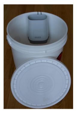
Warning, if you use this technique, you should drill a hole into the side of the bucket, just below the sensor, in order to assure that the sap doesn't drown and short-out the sensor. If you don't want to place the sensor into the bucket, you can custom make any sort of setup that keeps things dry. The key is that the sensor is fairly level, and over the bucket, since the sap drops out of the bottom of the sensor. The housing we use at howitrunning.com is shown below [without the roof].
